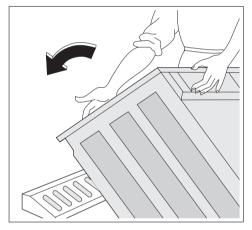
2. Remove the power supply cable and the draining and inlet hose from the hose holders on the rear of the appliance.
